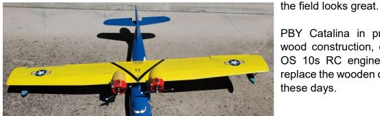
PBY Catalina in pre-war markings(?). All wood construction, doped and powered by OS 10s RC engines. 3D printed cowls to replace the wooden originals. Might fly one of these days.
